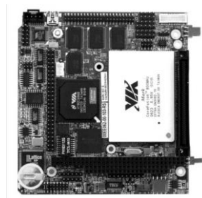
Figure 1. Athena II SBC Control System.
