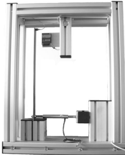
Figure 1 – Laboratory model with cantilever beam
