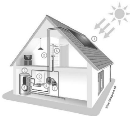
Figure 1. Basic concept of a solar water heating system for a family house.
